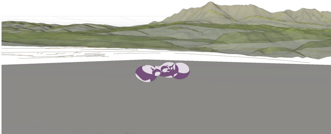
Fig. 7.7. Lateral 3D view of the Gardanne site, showing selected moment tensor solutions (focal spheres, back hemisphere projection) in the shallow underground (topography is exaggerated); similar sub-vertical pressure axes characterise the moment tensor solutions
